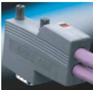
Other manufacturers like Delconec or FCT also provide CAN bus couplers. According to ISO 11898 Norm, Cable line impedance must be 120 Ω. For CAN cabling the use of twisted pair cable (2x2) having an impedance of 108...132 Ω is recommended.
