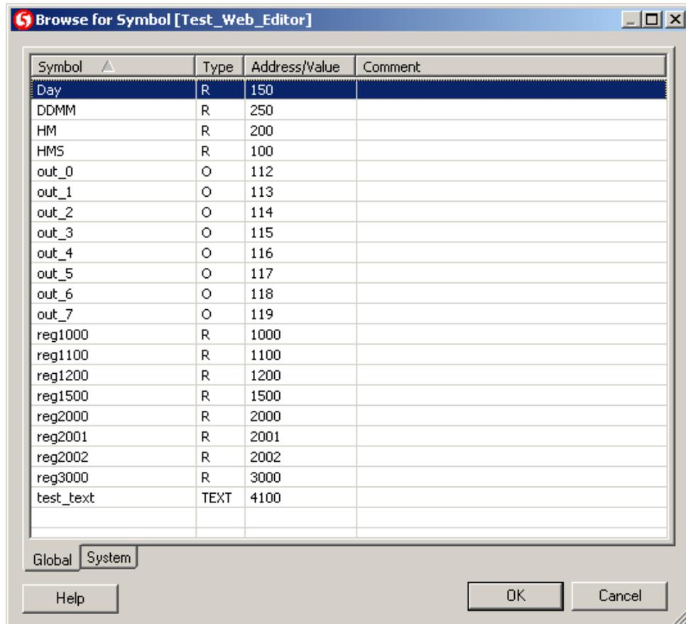
The 'OK' button of the properties dialog will then save these settings to the view. All the process points defined in the project can then be configured with the limits (min and max values), format and unit value (example °C) by opening the process point dialog using the menu Project ->Init PPOs... These process points are only linked with the relative addresses, which are the symbols defined in PG5, when a build is made of the whole project in PG5
