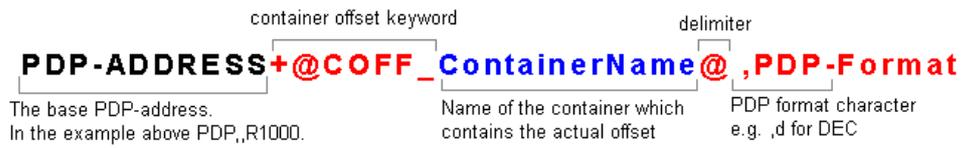
The text from the prefix '+@COFF\_' until the delimiter '@' will be replaced with the value of 'ContainerName'. It assumes the value of the container is an integer value.
