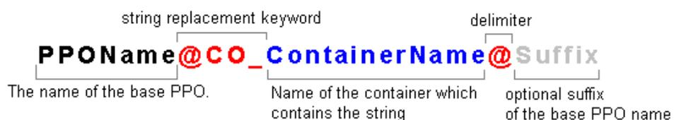
The text from the prefix '@CO\_' until the delimiter '@' will be replaced with the string in the container 'ContainerName'.
