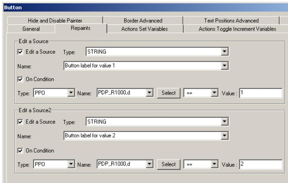
First you choose the type of the variable of which the condition shall depend. Choose 'PPO' for real process points or 'CONTAINER' for HMI-internal variables. Then indicate the name of the variable in the field 'Name'. Now you can set the value in the field 'Value' to which the variable shall be compared to and the type of comparison that can be:
