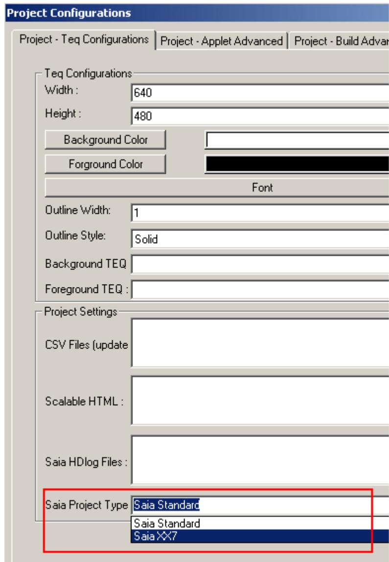
This step changes the project type and automatically replaces your IMasterSaia5\_15\_00.jar with IMasterXX7\_5\_15\_00.jar, which is the Java Applet that is specific to XX7 projects.
