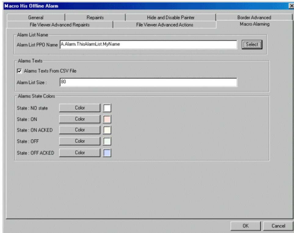
4. Click the 'Select' button next to the 'Alarm List PPO Name' text field to choose the PG5 symbol (e.g. A.Alarm.ThisAlarmList.MyName). By the PG5 symbol the Alarm Macro is referenced to the corresponding alarm list in the PCD.
