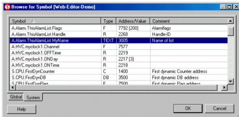
The PG5 symbol of the alarm list is automatically generated when using the Alarming FBox library. The user can define the Alarm list name by entering resp. modifying the name of the FBox.
