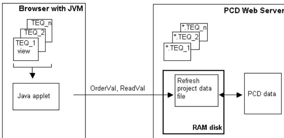
If the maximum number of PCD variables is exceeded in a given project, older firmware versions may cause the PCD to crash. In systems with new versions, all PCD variables are no longer refreshed, and a "No message" error will be displayed in the browser. There will also be an entry "WEB RAM TOO SMALL" in PCD history.
