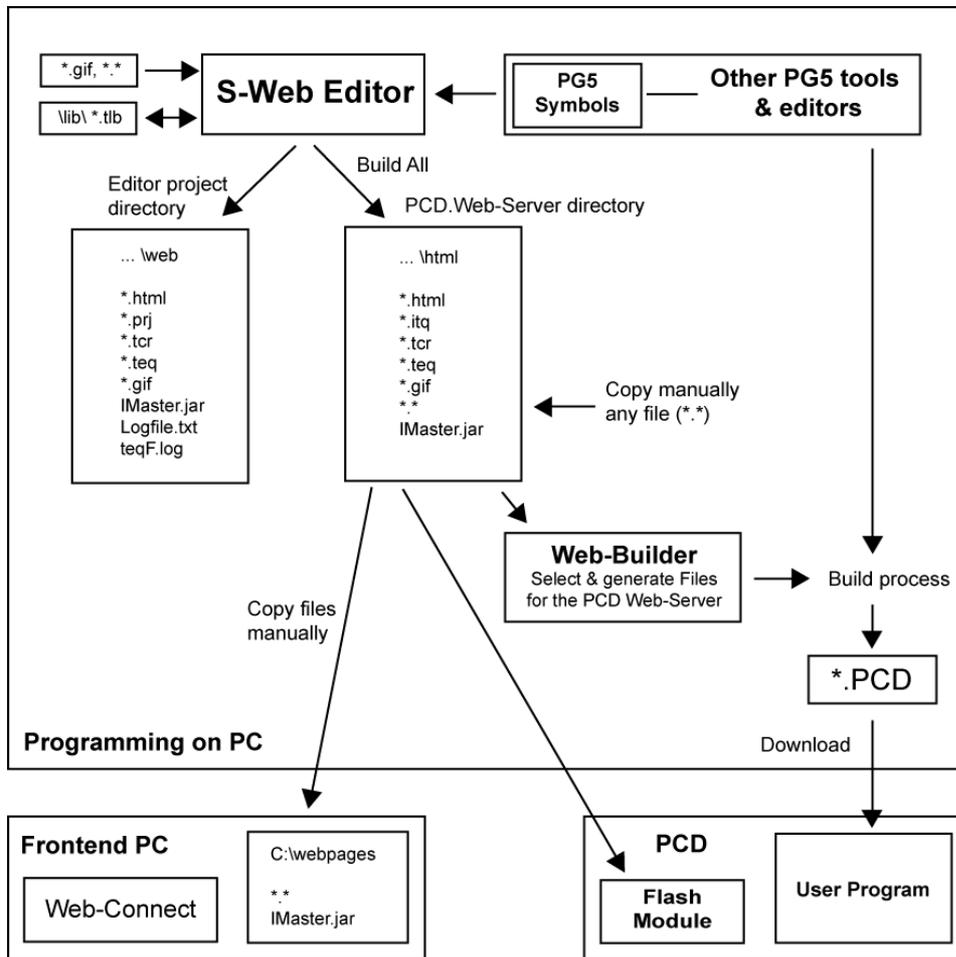
This section explains the project structure and the files which are necessary to produce a Saia®PCD.Web-Server application with the Web-Editor.
