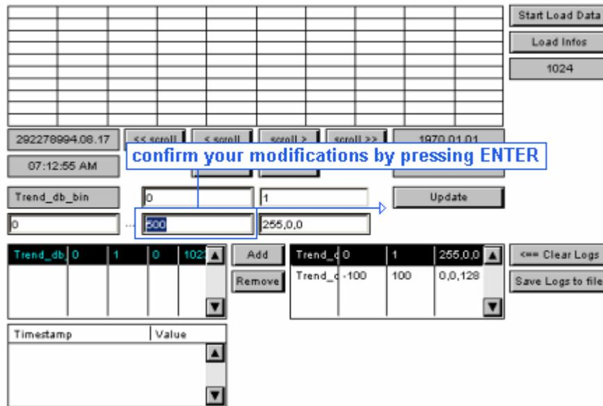
Click "Start Load Data" to initialize the upload process. If the upload takes too long, this process can be interrupted by pressing the button 'Stop Loading'. The data that was loaded so far is not lost.
