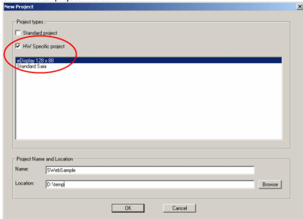
According to the hardware profile the project wizard will make the project settings that fit best to the eDisplay hardware (TEQ-View Size, zoom factor, colour...etc.). S-Web Editor automatically sets the recommended project settings for the eDisplay hardware.
