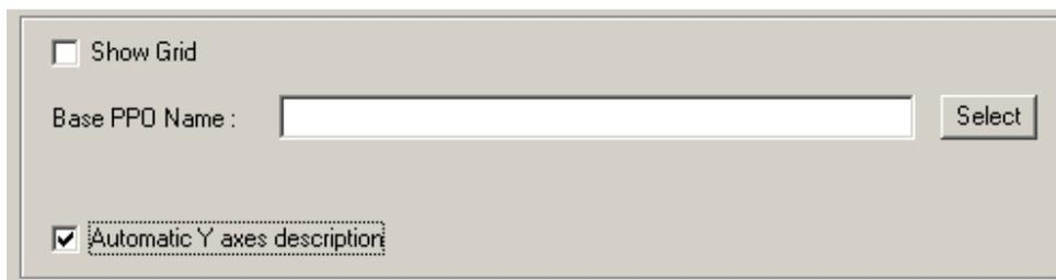
"Automatic Y axes description" will add a description for each curve to the y-axis at runtime. The description shows you a scale from the defined "Y Min" to "Y
