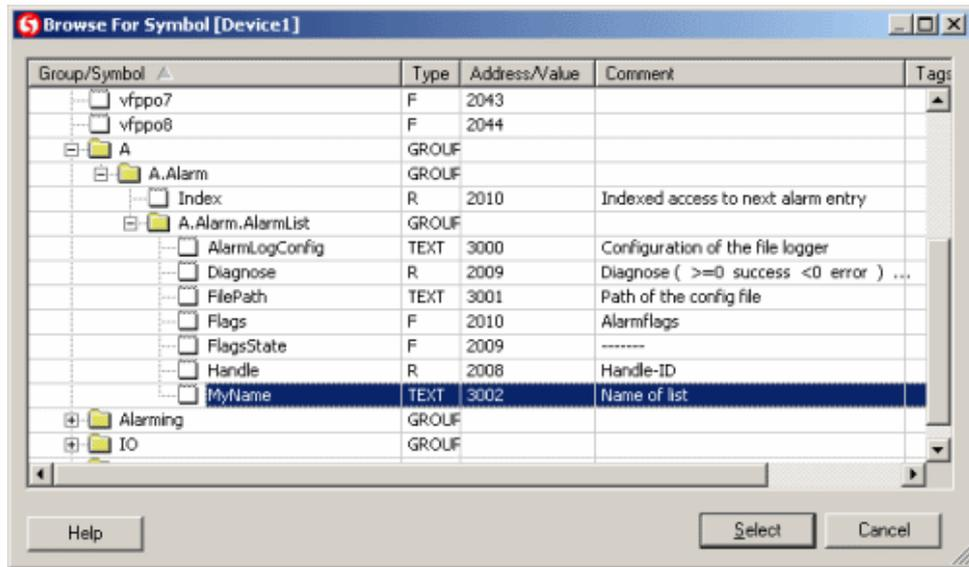
(After configuring this PPO, the event list macro is connected to the corresponding object instance in your PG5 program.)
