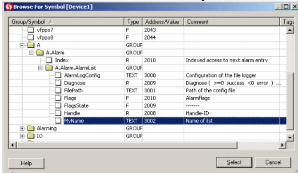
(After configuring this PPO, the alarm list macro is connected to the corresponding object instance in your PG5 program.)
