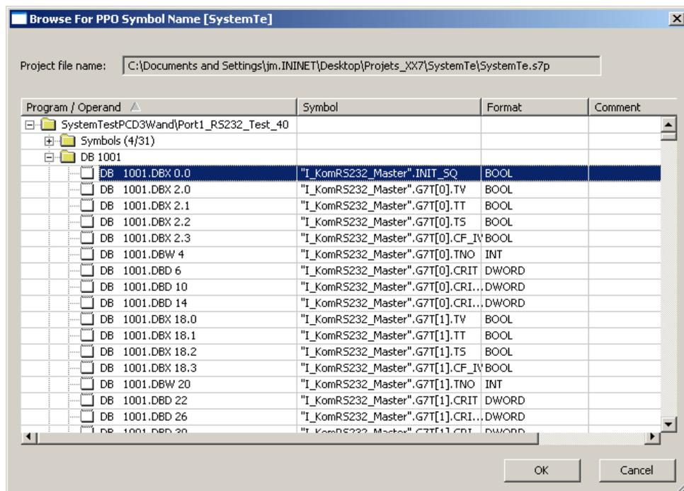
Additionally, it is also possible to use container offset inside XX7 symbols. This is very useful when accessing your S7 data arrays and even arrays of structures with the help of container variables.
