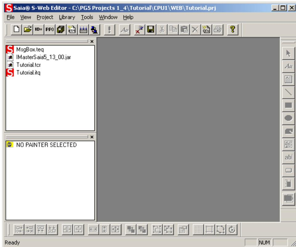
This is the main window of the S-Web Editor application. It controls all the other windows and is used to do basic settings. All files belonging to this project will be added to the PG5 project under a sub directory called 'Web'.
