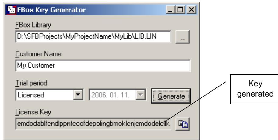
In the FBOX Library field should be filled by default if Key Generator is opened from FBOX Builder and it should display the full path of the LIN file of your active library. The path of this LIN file is the following:
