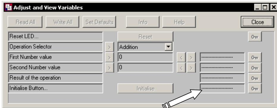
3. Add a string corresponding to the "0" state of the static flag that belongs to the Button with View. Open the properties dialog window and modify it as follows:
