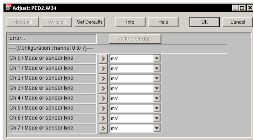
The structure of this dialog is defined by the AV entries of the definition file; but the text displayed are defined in the "FBOX Display Texts" (.IDX file) which we will see the details in the next paragraphs.
