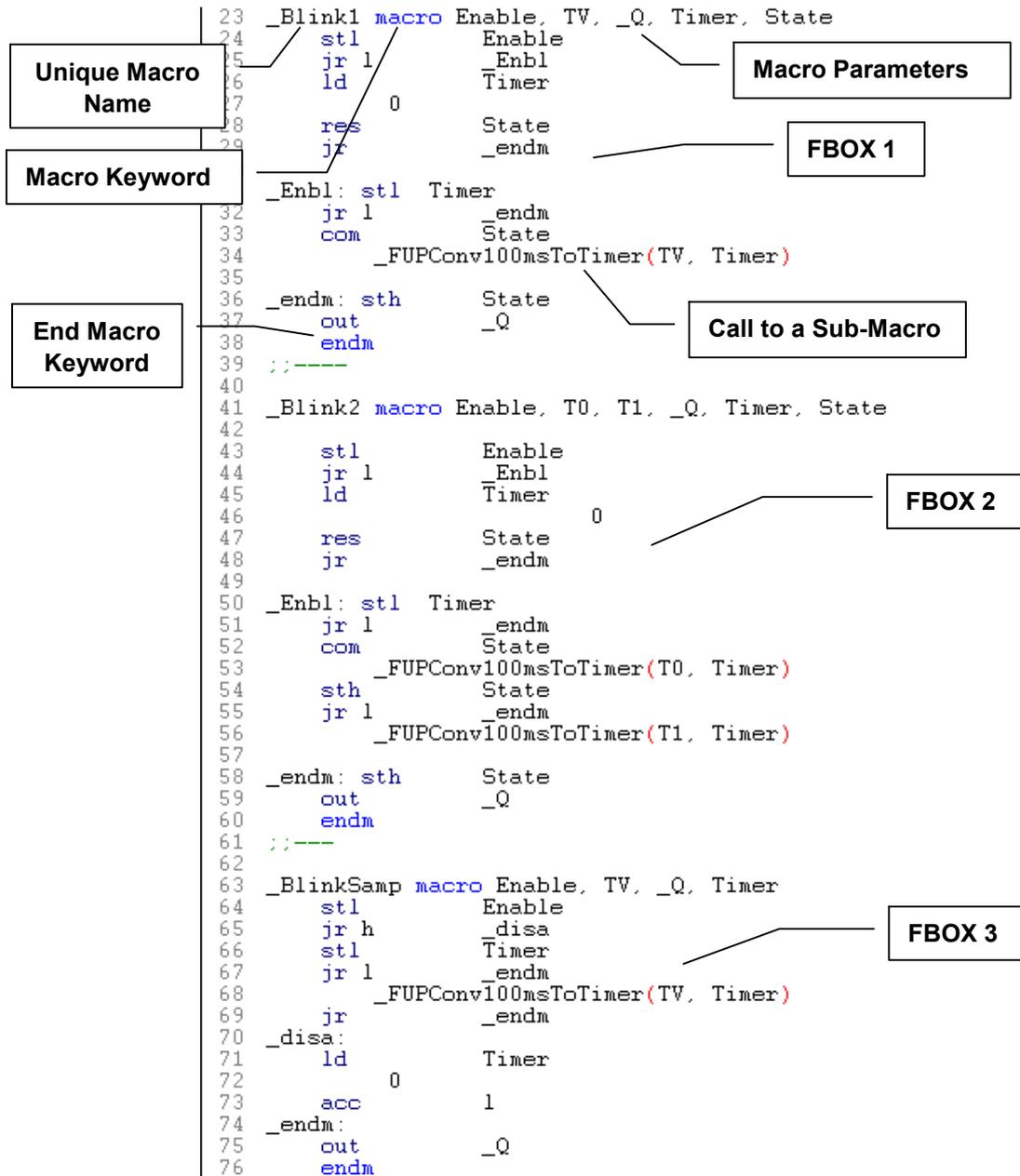
The macro name of each FBOX must be exactly the same as the one of the definition file. As you can see on the above picture, each macro has parameters. The definition of each FBOX defines the parameters of the macro. The FBOX Builder generates the macros only based on the definition information. The order of the parameters is very important; we'll see in details in this chapter what these parameters are linked to.
