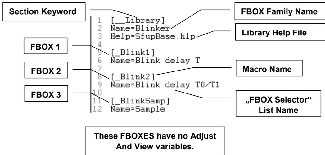
Like with the “.LIB” file described in the previous paragraph, the macro name of each FBOX of the “.IDX” file must strictly correspond to the one defined in the definition file. The FBOX Builder can generate this file.
