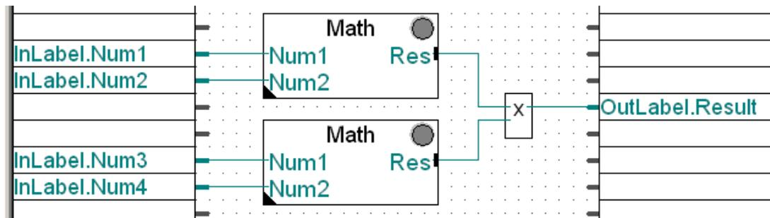
The Adjust dialog of each “Math” FBOX stays unchanged that means each “Math” FBOX does a simple addition between “Num1” and “Num2”. The results of both of them are finally multiplied.
