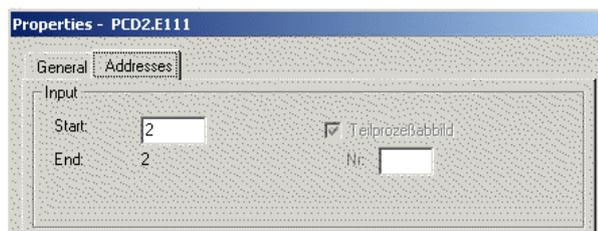
If the address range for the digital input modules is between 0 and 255, the input will be read cyclically and copied to the process map.
