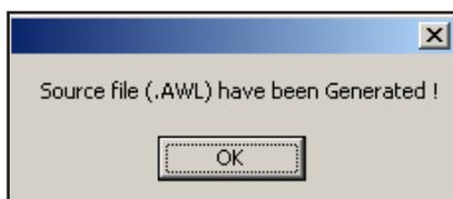
When the AWL source has been successfully generated, it is ready to be imported into STEP®7.
