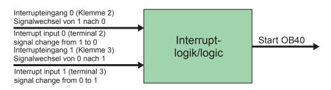
OB40 processing can determine at which input the interrupt was triggered. This is done by analysing the local data byte "OB40-SRT-INF". The following mapping applies:
