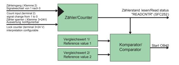
SFC251 (INTCNTR) is used to configure and start or stop the unidirectional counter. A single SFC251 call in the application program is sufficient to configure / start the counter.
