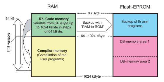
The DB memory area must be partitioned, to prevent "over-filling" the Flash EPROM. This would occur relatively quickly, as old DB versions in Flash EPROM are not deleted but simply marked as no longer valid.
