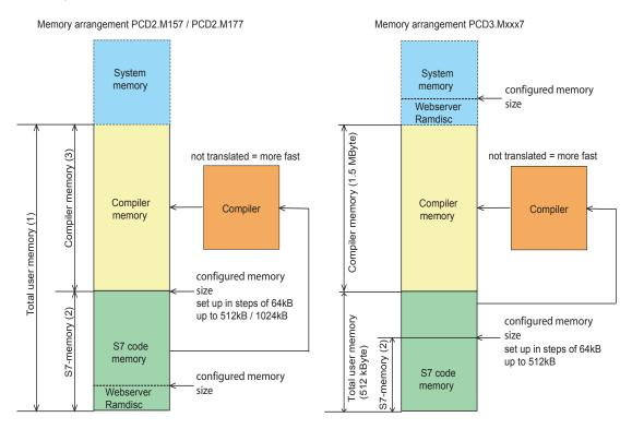
The PCD2.Mx57, M177 and PCD3.Mxxx7 controllers have the capability to compile the application program. In contrast to interpreted code, where every command is translated from scratch at run time, compilation translates these commands into "CPU-language" before the execution of the program. By eliminating the translation
