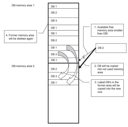
If a DB is larger than the available memory area, it will be copied together with current DBs to the second DB area. The whole DB area with the old DBs will then be deleted, releasing the memory.
