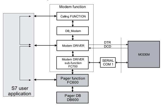
The Pager function is associated with a Pager Data Block. The Data Block is divided in two areas. One is reserved for internal use of the function and the other area contains the information about the application. The Pager function also needs to access the sub-function of the FC700 (Modem Driver sub-function).
