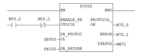
When the function is executed once, the protocol is enabled if no error was done in the configuration parameters, then the output **PROTOCOL\_ON** is set to 1. If an ER-ROR happened during enabling the protocol, the output **ERROR** is set, the **STATUS** includes the error code.
