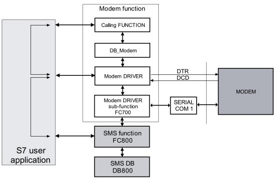
The SMS function is associated with an SMS Data Block. The Data Block is divided in two areas. One is reserved for internal use of the function and the other area contains the information about the application. The SMS function also need to access the sub-function of the FC700 (Modem Driver sub-function). The synchronization between the Modem Driver and the SMS function is made by the S7-application.
