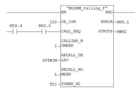
As soon the connection is completed, the Driver signals it by setting the bit M50.2 to 1 and as it is an outgoing call the bit M50.3 stay at 0.
