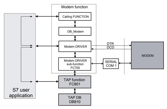
The TAP function is associated with an TAP Data Block. The Data Block is divided in two areas. One is reserved for internal use of the function and the other area contains the information about the application. The TAP function also need to access the sub-function of the FC700 (Modem Driver sub-function). The synchronization between the Modem Driver and the TAP function is made by the S7-application.
