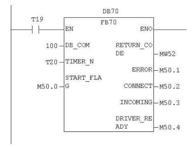
On the POWER ON or on the STOP  $\rightarrow$  RUN phase, all the non-retentive flags are resetted, so we are sure that, when we call the FB70, the input START\_FLAG (M50.0) is 0. This will start the Driver and initialize the modern. After the first execution of the FB70 the flag M50.0 is set to 1. As soon the modern and Driver are ready the flag M50.4 is 1.
