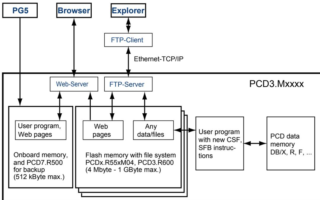
FTP server and file system access can only be achieved with the plug-in flash memory module. Access via FTP server is only possible via the Ethernet TCP/IP interface.
