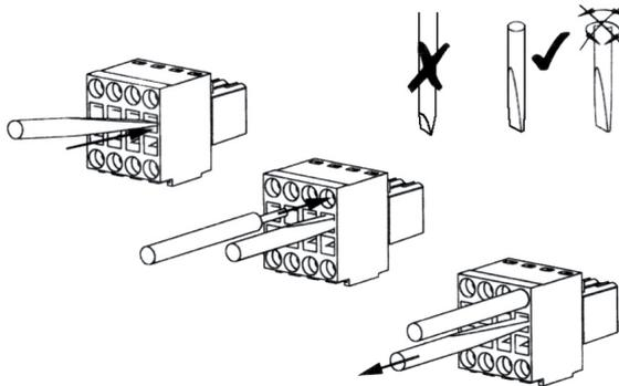
The plug-in cage clamp terminals simplify the installation significantly. The cage clamp terminals support cable diameters from 1.0 mm<sup>2</sup> through 1.5 mm<sup>2</sup> up to 2.5 mm<sup>2</sup>.
