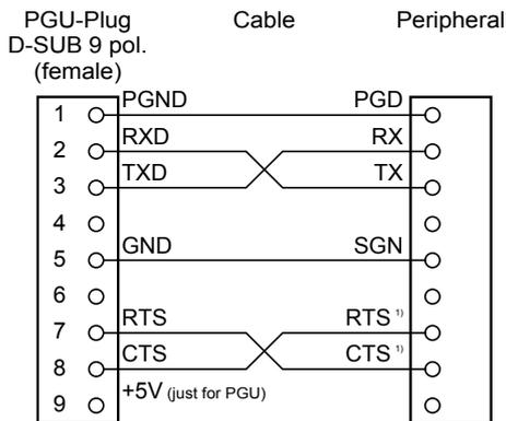
1) When communicating with terminals, check whether some connections are provided with bridges or need to be set to "H" or "L" with the "SOCL" instruction. It is generally recommended to use a handshake (RTS/CTS).
