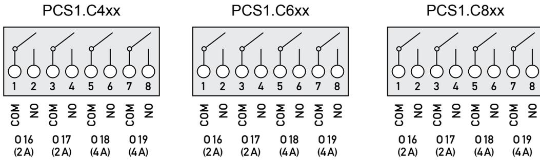
**5.4.2 Digital relay outputs with change-over contacts, terminal block X8**
