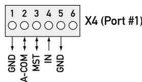
Up to 8 MFT/MFT2 drives from BELIMO® can be connected to the PCD7.F180 connection module for the MP-Bus. For details see Technical Information P+P26/342.
