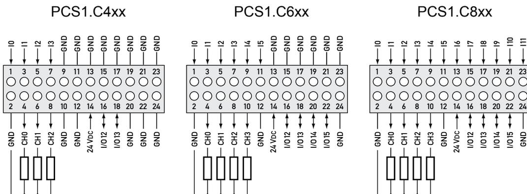
Connection example: fan drive with analogue output
