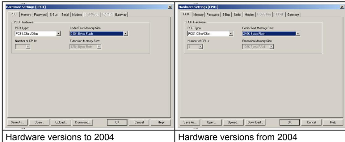
There are only 128 kB of flash EPROM available for code/text memory. One block of memory is lost to configuration data (header), because flash EPROM can only be accessed in block mode.
