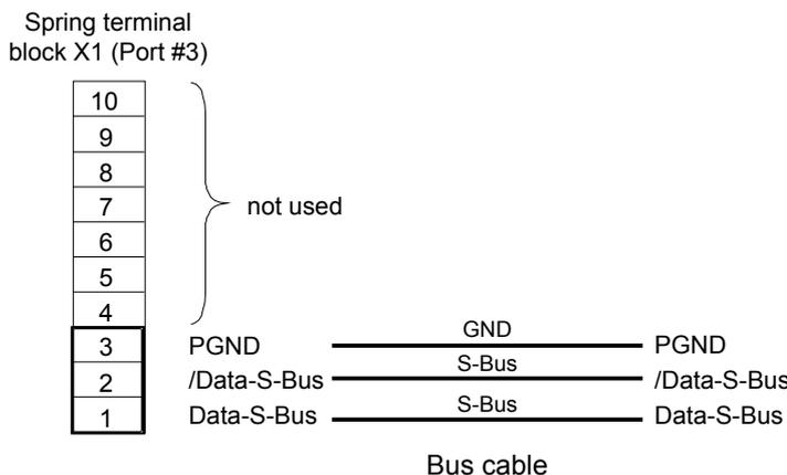
**Connecting communication interfaces with RS-485 to X1:**
