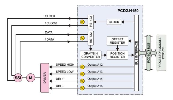
As the block diagram shows, the SSI encoder is capable of direct connection.
