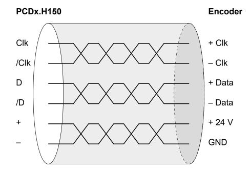
To prevent interference problems, a shielded and twisted pair cable should be used and the shield should be connected to ground on both sides.
