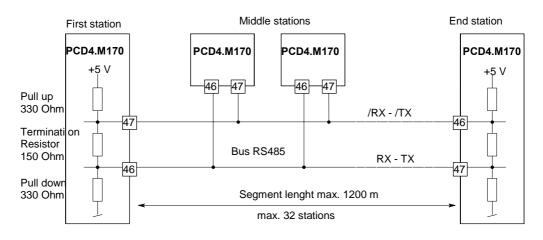
**Note:** It is recommended that the line termination resistors should be included in the cable connector. There are no termination resistors on the module itself.
