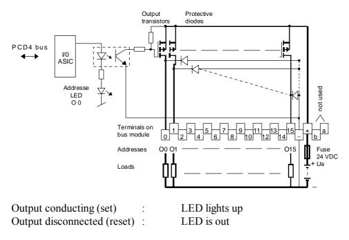
The minus terminal (-) is NOT connected to the internal ground. Due to interference decoupling capacitors on the bus module from - and + terminal to PGND, the common mode voltage is limited to 200 V AC or DC.
