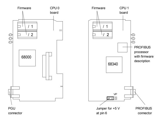
The three types of firmware for the CPU 0, CPU 1 and for the PROFIBUS-FMS co-processor must co-ordinate with each other. Therefore any firmware updates should only be carried out in the factory.
