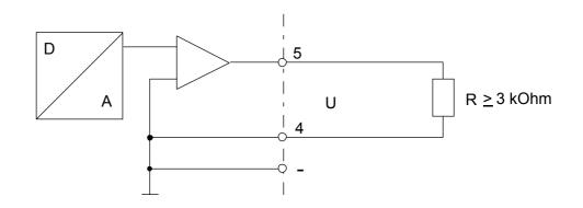
• Current outputs for range : 0 ... 20 mA or 4 ... 20 mA (selectable with jumpers)
