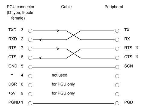
1) When communicating with terminals it is necessary to check whether certain pins should be provided with bridges, or whether they should be set H or L with the SOCL instruction.
