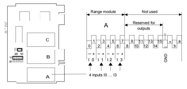
Installing at space A <u>Range module</u> PCD7.W105 : measuring range 0 ... 20 mA, 4 ... 20 mA, ±20 mA or ±10 mA
