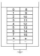
The terminals are always numbered from 0 ... 15. The absolute output address is determined by adding the basic address of the module to the terminal number.
