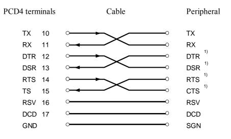
Adapt connector type and connections according to the peripheral.
