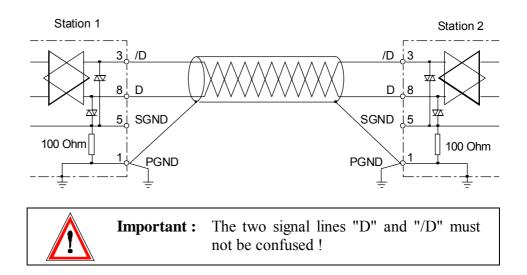
For the wiring diagram shown above, the potential difference between the data reference potentials SGND of all stations should not exceed  $\pm 7$  V.
