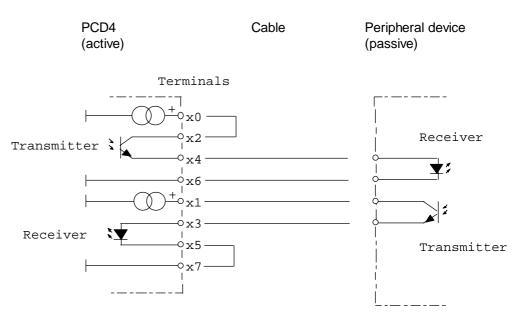
\*) max. baud rate for 20 mA current loop limited to 9600 Baud
