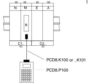
5) Connect 24 VDC smoothed or 18 VDC full wave rectified to terminals + and –. For small-scale requirements, 24 VDC at 0.5 A is adequate. An easy way to do this is to use the PCA2.SO5 input simulator (no longer available), which not only provides 16 input switches but also offers 24 VDC.
