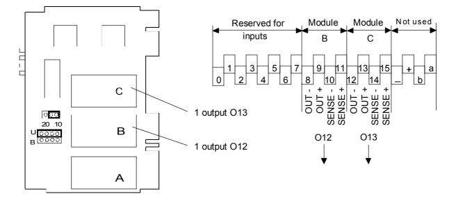
Installing at space B and/or C
