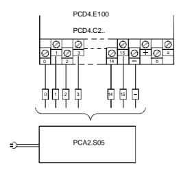
• Connection of PCD8.P100 programming unit
