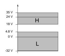
Due to the input delay of typically 9 ms in the standard version (...B900), full-way rectified DC voltage is adequate for the external supply.
