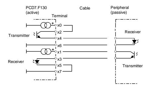
\*) max. baud rate for 20 mA current loop limited to 9600 Baud
