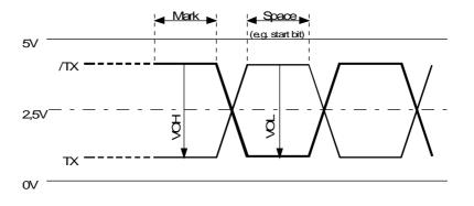
VOH = 2 V min (with load) to 5 V max (without load) VOL = -2 V ... -5 V
