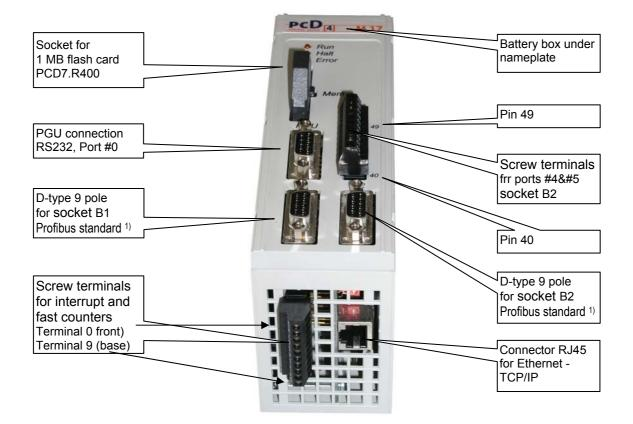
1) The pin configuration of these two D-Sub connectors (9 pole female) complies with the PROFIBUS standard. The two D-type connectors should preferably be used for PROFIBUS networks. Further serial ports should, if possible, be connected to the 10-pole plug in screw terminals.
