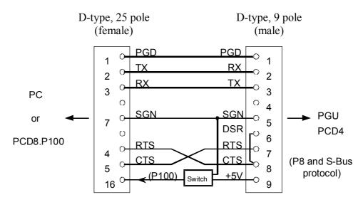
**PCD8.K101 connecting cable** (for P8 and S-Bus protocol) (as replacement for ..K100 which cannot be used for PCD1)
