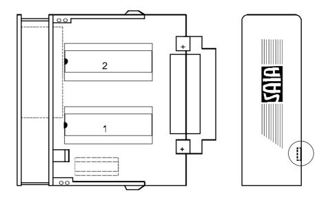
The memory module is provided with a security clip to prevent it from falling out during transportation and heavy vibrations. To remove the module screwdriver no. 1 or 2 is needed. The screwdriver must be inserted and the memory module simultaneously removed.
