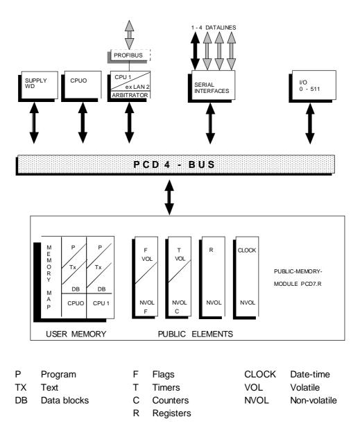
The following block diagram shows the internal structure of the PCD4 system :
