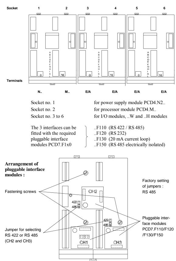
The PCD4.C340 bus module has 6 sockets :
