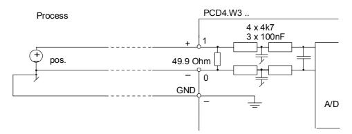
Note: The process ground, or that of an input amplifier, must be connected to the ground of the analogue module (at terminal " – "). Instead of a separate ground line the shield of the cable can be used.
