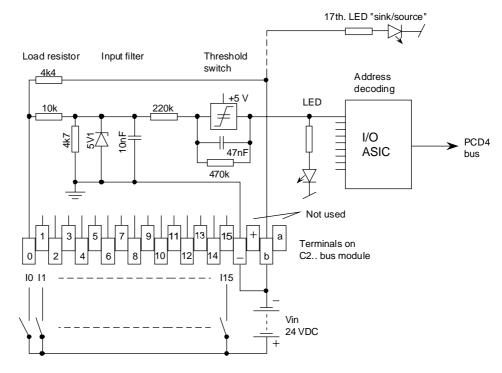
• Source operation or positive logic : (for standard version 24 VDC)
