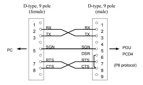
PCD8.K111 connecting cable (for P8 and S-Bus protocol)
