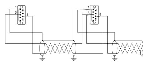
Care should be taken to ensure that the bus line still remains continuously connected when one or more plugs are removed.
