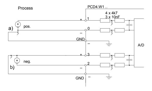
Note: The process ground, or that of an input amplifier, must be connected to the ground of the analogue module (at terminal " – "). In unipolar operation, the more positive potential is connected to the " + " terminal. In this way, negative voltages (b) can also be measured.
