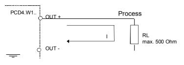
For supplying current outputs, the "+" terminal must be connected to +24 VDC. This supply can be that same as that of the power supply module PCD4.N2.. with a maximum current requirement of 60 mA.
