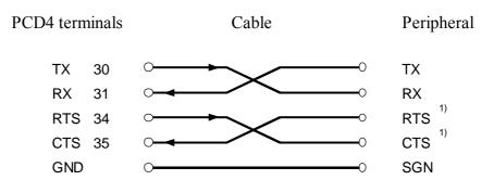
Adapt connector type and connections according to the peripheral.
