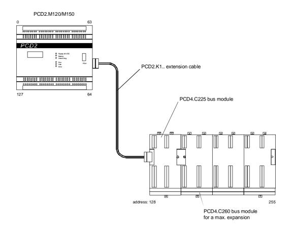
As with a PCD2.C100 expansion unit, addressing of the PCD4.C225 starts at 128 and extends, if fully equipped with a maximum of 8 modules, to 255. If an attempt is made to fit a 9th module, addressing starts at zero and then runs parallel to the address range of the PCD2.M... base module (addresses 0 - 15).
