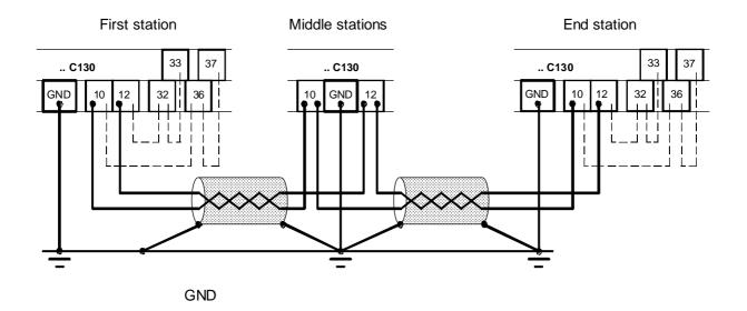
It is recommended that the RS 485 cable is not laid in direct proximity to motor cables which may produce interference, unless these cables are also well screened.
