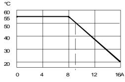
Mean sustained overall current for all outputs in the same module (module in vertical position)
