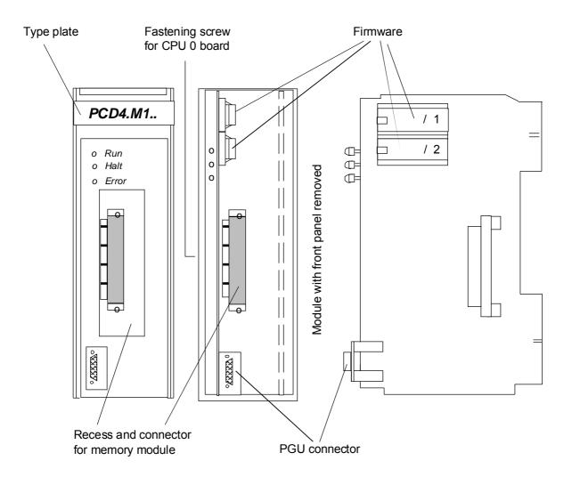
To update the firmware, remove the processor module (cartridge) from the bus module, then remove the front panel from the processor module and unscrew and take out the board. Now both EPROMs can be easily changed. Re-assembly is done in the reverse order.
