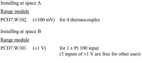
The 2 mA constant current for the resistive temperature sensor Pt 100 is supplied by the RTD+ terminal.
