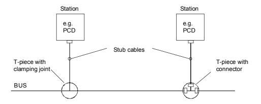
In the case of a wiring plan using stub cables, care should be taken to ensure that the shielded stub cables are no longer than 100 cm for a transmission speed up to 19.2 kBit/s, and no longer than 30 cm for 500 kBit/s.
