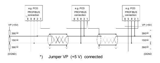
The PCD7.T160 termination boxes should be used to terminate the bus cleanly :
