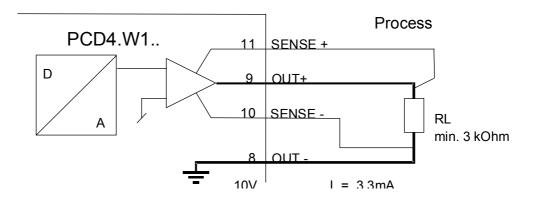
**Note :** Two "SENSE" measurement cables are provided to increase voltage precision at the load resistance RL.
