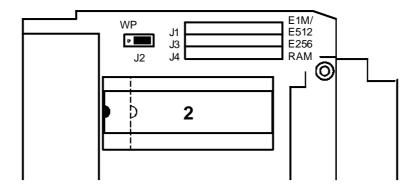
Insertion of jumpers allows the following memory chips to be fitted :
