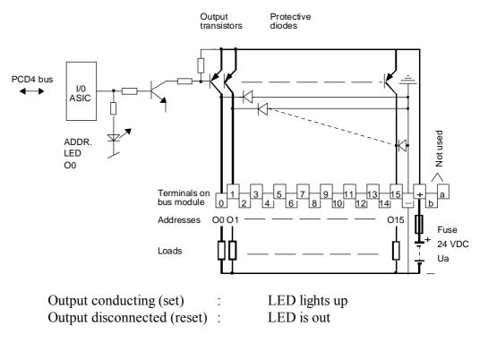
Fuse : It is recommended that each PCD4.A400 module is protected against short-circuit with a quick-break fuse of max. 10 A.
