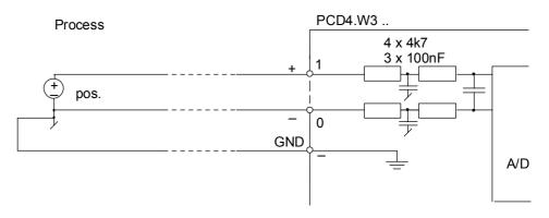
Note: The process ground, or that of an input amplifier, must be connected to the ground of the analogue module (at terminal " – "). Instead of a separate ground line the shield of the cable can be used.
