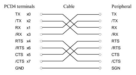
Adapt connector type and connections according to the peripheral.
