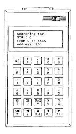
The LCD-Display has a backlight to produce optimum contrast whatever the lighting conditions. The contrast and reading angle can be adjusted by inserting a screwdriver into the opening next to the connector.
