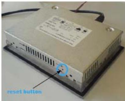
C. Then at the same time Power ON the MB-Panel. Wait about 3-4 sec. until the LED is flashing. Then Download the FW with the Saia firmware download utility.
