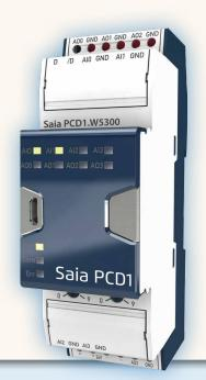
Inputs 4× analogue 0...10 V, ±10 V, ±20 mA, Pt / Ni 1000, NTC, KTY, 0...2,5 kΩ, 0...7,5 kΩ, 100  $\Omega$ ...100 kΩ
