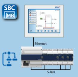
Connection to web panels via PCD controllers also functions smoothly. Automation systems have the crucial advantage of requiring little space and being switchbox-compatible
