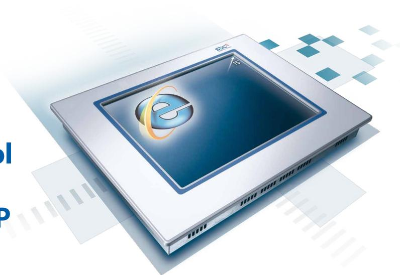
The Saia PCD7.D6150TA010 series Web-Panels are specially designed for the needs of web visualisations, and are pre-configured with all the applications and software tools needed for this. No need for complex installation and software updates – Saia PCD® PCD7.D61xxTA010 series Web-Panels are ready for use right away. The Web Panel eXP has a display size of 15" with XGA resolution 1024 × 768 pixels.
