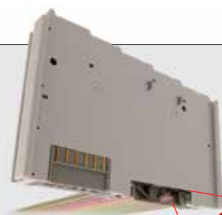
The Achilles' heel of the system: the ground connection of individual bus terminals on slice.
