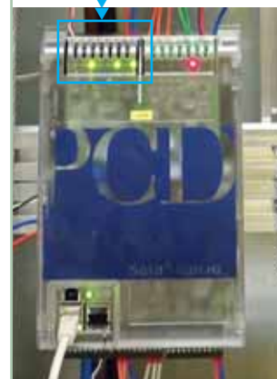
▲ Saia®PCD1.M2120 with M-Bus module
