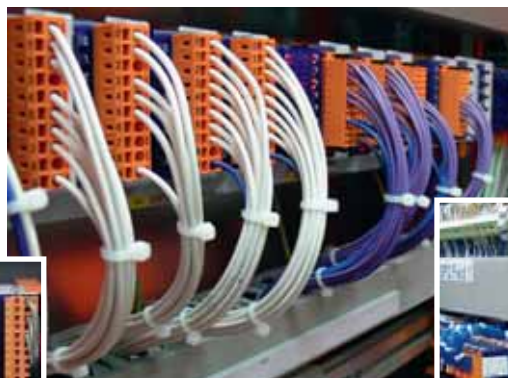
▲ Saia® PCD3 with I/O module for conventional sensors/actuators
