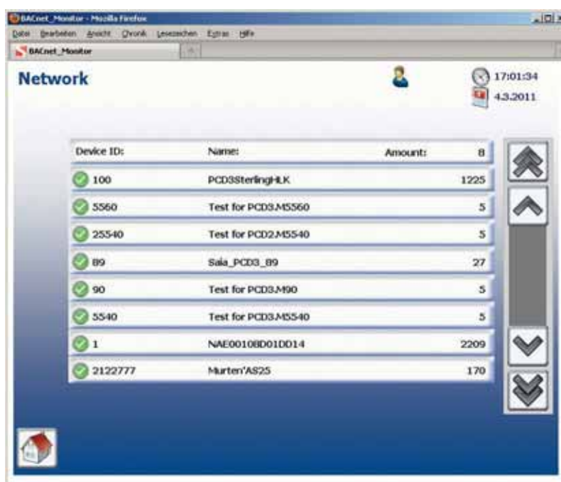
▲ BACnet devices are presented in a user-friendly way. Image: a test facility with controllers by JCI, Saia®, Sauter and Siemens.
