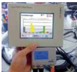
▲ Saia® Functions HMI as KSB PumpManager with the KSB PumpMeter in the KSB Development Centre.
