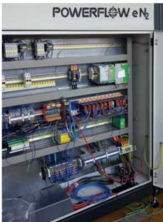
▲ Powerflow eN 2 Compact full tunnel wave soldering machine with Saia® PCD
