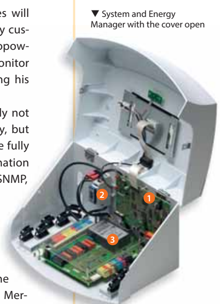
1 Standard Saia®PCD CPU board 2 1-phase Saia® energy meter 3 Vaillant-specific I/O board
