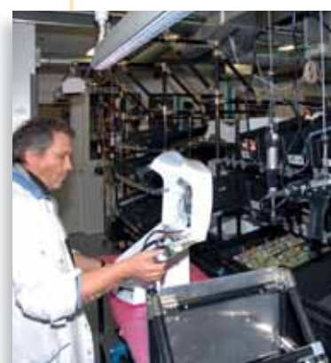
▲ System and energy manager assembly line for the Vaillant-Honda micro-CHP system: The Saia® boards are assembled and tested according to lean methods on the production line created for this product
