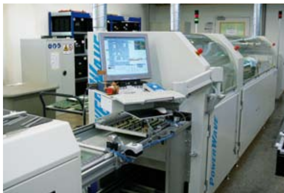
New wave soldering machine for the leadless soldering process
