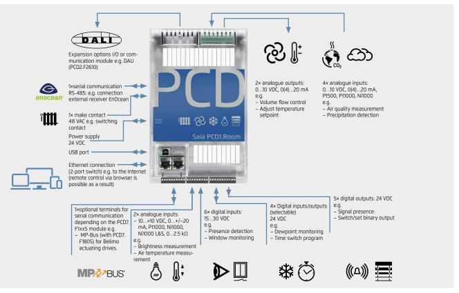
Lighting, sun protection and individual room regulation can be optimally coordinated with one another with this controller. This example showing possible assignments was compiled based on applications in accordance with the VDI 3813 list of room automation functions and the DIN EN 15232 list of building automation functions.
