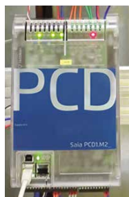
Use as communication interface with M-Bus in a district heating network
