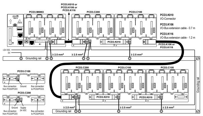
The PCD3.C200 module holders provide the following internal supply currents to the modules plugged in or connected to them:
