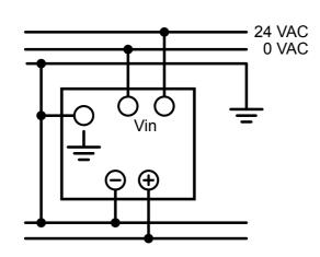
Output: Output voltage 24 VDC is made via the positive (+) and negative (-) terminals. The red LED DC signalises the correct output power. When the red LED is blinking, the device is in overload range or in short circuit protection.
