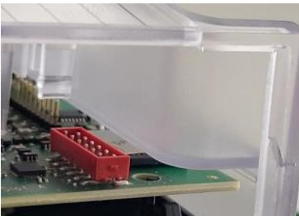
Push with a screwdriver the black lower part of the housing to the left side, so that the nose will move to the left and the PCB snaps again to the black lower part of the housing.
