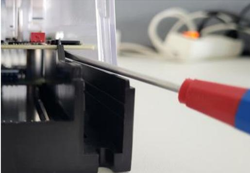
With the thumb of your left hand, lift the PCB for about 3 mm
