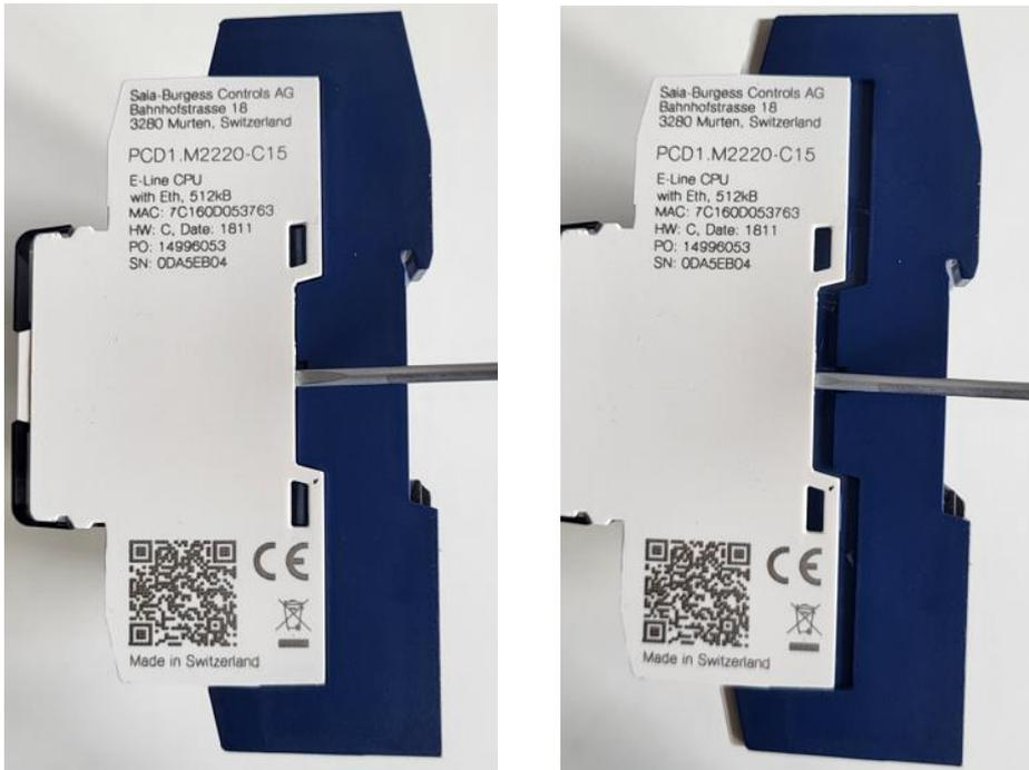
Push the screwdriver slightly upwards until the 2 holding noses located on the blue housing base are no more located on the 2 rectangle holes located on the white upper part of the housing.
