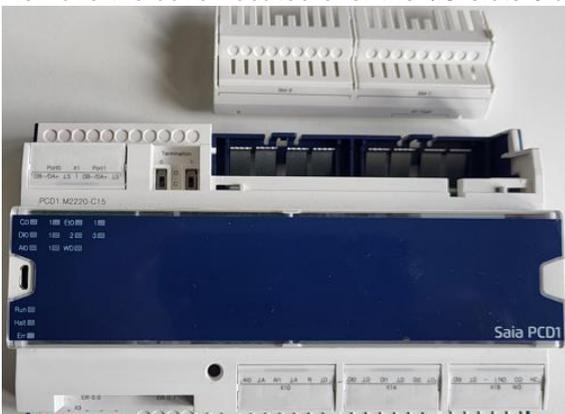
Insert a slotted head screwdriver 2.5 x 50 on the appropriate position on the right side of the housing and push the screwdriver for ~ 3 mm under the white upper part of the housing.
