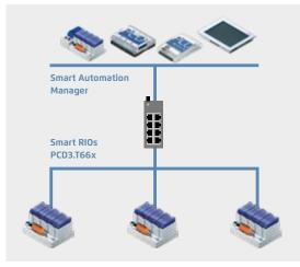
As Smart Automation Managers, PCD1.M21x0, PCD2.M5, PCD3.M2/3/5 CPUs and the programmable micro browser panel PCD7.D4xxxT5F can be used
