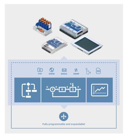
▲ Functional structure of Saia PCD<sup>e</sup> control units: The entire automation application is onboard. The combination of globally standardised, non-proprietary Web+IT functions known as Automation Servers form the interface to the environment. The fully programmable design and modular expansion of the controller ensure the "perfect fit" for current task formulation over a service life of 15-20 years with no need for new investment. 243
