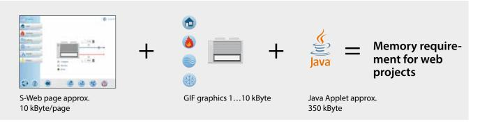
A project with 30 HMI pages will therefore need approx. the following memory requirement: (30 × 10 kByte) + (100 × 5 KByte GIF graphics) + 350 kByte = memory requirement for web project approx. 1150 kByte
