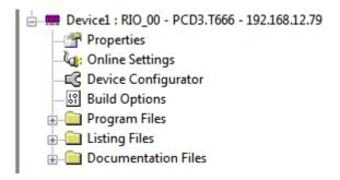
From there, you can add program files to the RIO, as for a PCD device – Fupla, IL, Graftec. User program data exchange between RIO and manager can be define using the RIO Network Configurator, selecting the corresponding RIO in the 'Media Mapping' view and selecting the 'New Data Transfer Array …' command of the context menu.
