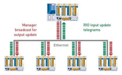
Efficient data interchange with the Ether-SIO protocol
