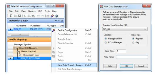
The transfer array can be specified by selecting the transfer direction, the data type, the size and the symbol name. Once done the transfer will be displayed in the 'Media Mapping' view, under the corresponding RIO.
