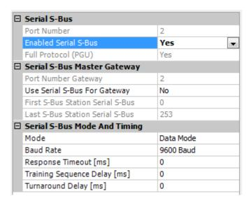
Modem, Profi-S-Bus, Ethernet and all gateway type can be configured in the same way.
