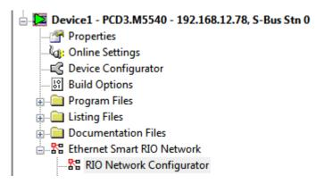
It is now possible to define RIO devices into the project with a double click on the 'RIO Network Configurator' item. The double click will open the 'RIO Network Configurator'. This is a new configurator especially developed for configuring the Smart RIOs. New RIO devices can be added using the 'New RIO ...' command from the 'RIO' menu.
